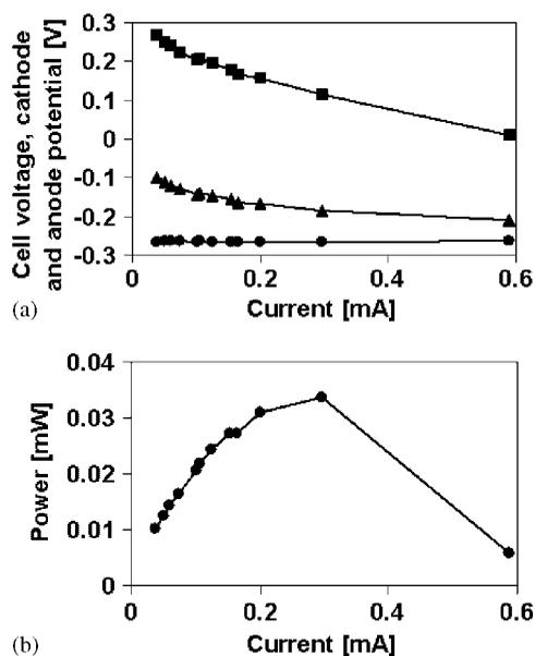
Figure 3. Polarization curve (a) with cell voltage (squares), cathode potential (triangles) and anode potential (circles); power curve (b) of plant-MFC no. 6 on day 90.
