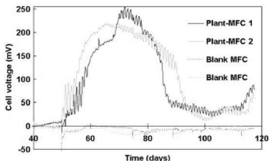
Figure 2. Plant-MFC proof of principle. Cell voltage (mV) of two plant-MFCs and two blank MFCs.
